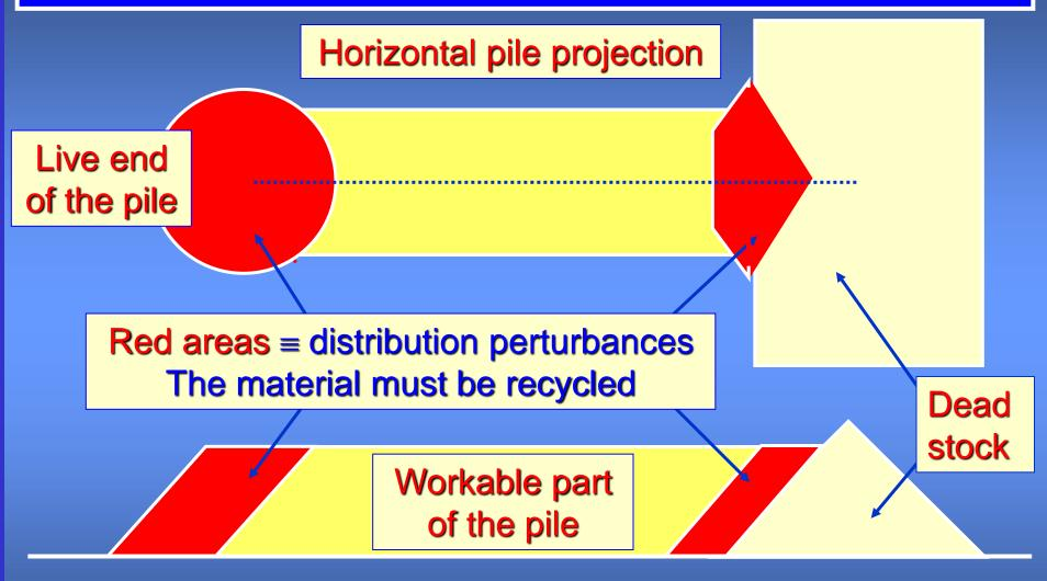
Vertical pile cross-section
